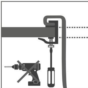
NOTE: do not use power or pneumatic screwdrivers which do not have load adjusters.
